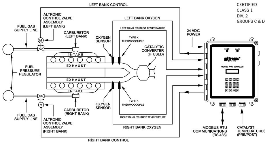
Setpoints are tied to one of two NC switch outputs for integration with a safety shutdown panel or supervisory control system. The Error Alarm Output is tripped for all setpoint violations associated with rich/lean control limits, oxygen sensor issues, and other values related to the control functionality. All catalyst temperature setpoint violations (pre-, post-, and differential) prompt the Catalyst Temperature Output to trip.
