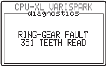
Too many or too few gear tooth pulses are seen between reset pulses. The received number of pulses is displayed.
