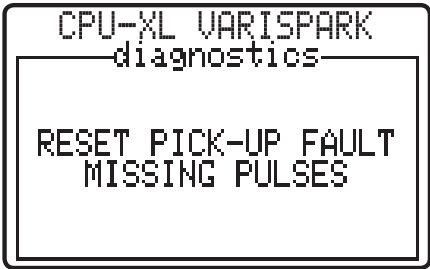
Too many gear-tooth pulses are seen without a reset pulse.
