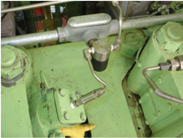
Pneumatic air distributor with pilot-actuated air-in-head valve
