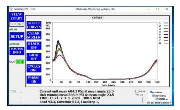
The screens above shows the phased and un-phased cylinder pressure plots. Combustion statistics that are tracked (and can be alarmed on) include:
