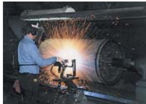
**Thermex®—Thermal Spraying**—Exline selects from hundreds of metallic and nonmetallic coating options and five thermal spray processes to achieve the surface characteristics you require, such as abrasion resistance, lubricant retention, and corrosion protection.
