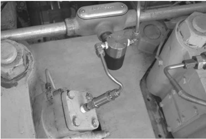
Pneumatic air distributor with pilot-actuated air-in-head valve
